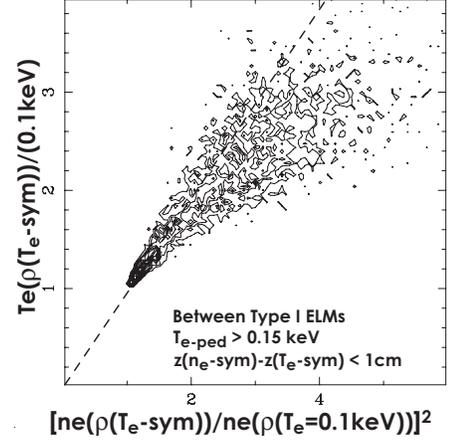
FIG. 4: Probability contours from DIII-D pedestal database (9104 points) of  $T_e$  versus  $n_e^2$  at  $\rho_T$ , referenced to their values at the point where  $T_e$  is 0.1 keV. Dashed line indicates  $\eta_e = 2$ .
