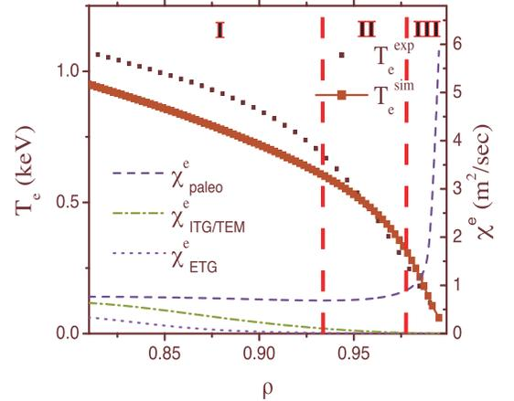
FIG. 3: ASTRA modeling (500 radial points) [18] of  $T_e(\rho)$  in H-mode edge pedestal like that in Fig. 1. Diffusivities due to ion-temperature-gradient/trapped-electron and electron-temperature-gradient microinstabilities are  $\chi_{\text{ITG/TEM}}^e$  and  $\chi_{\text{ETG}}^e$ . Edge (regions II,III)  $T_e$  profile is determined by  $\chi_e^{\text{pc}}$ .
