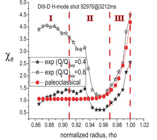
FIG. 2: Interpretive [16] profile of  $\chi_e$ ,  $\chi_e^{\text{pc}}$  ( $\text{m}^2/\text{s}$ ) in pedestal similar to Fig. 1. Agreement in edge (II,III) is reasonable since uncertainties in both  $\chi_e$  values are  $\gtrsim 2$ .  $(Q_E/Q)_{\text{sep}}$  is assumed electron fraction of power flow through separatrix.
