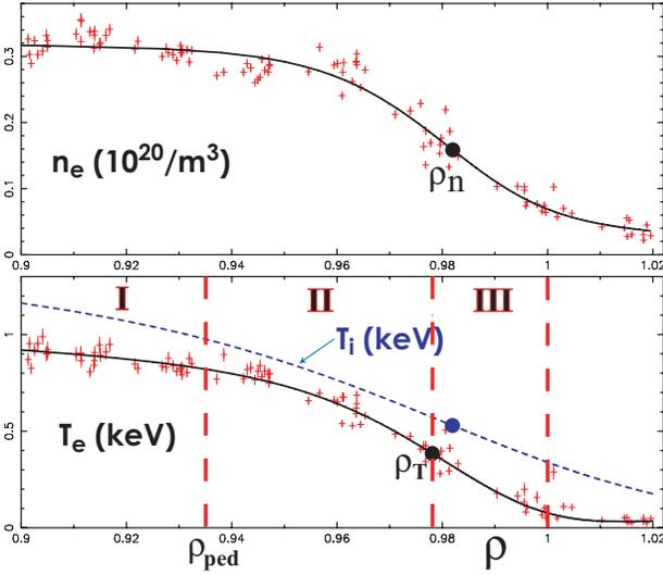
FIG. 1: “Equilibrium”  $n_e$ ,  $T_e$  pedestal profiles for DIII-D H-mode shot 98889, averaged over 80–99% of time ( $\sim 36$  ms) to next ELM crash, around 4500 ms. The lines show tanh fits to Thomson scattering data with symmetry points at  $\rho_n$ ,  $\rho_T$ .
