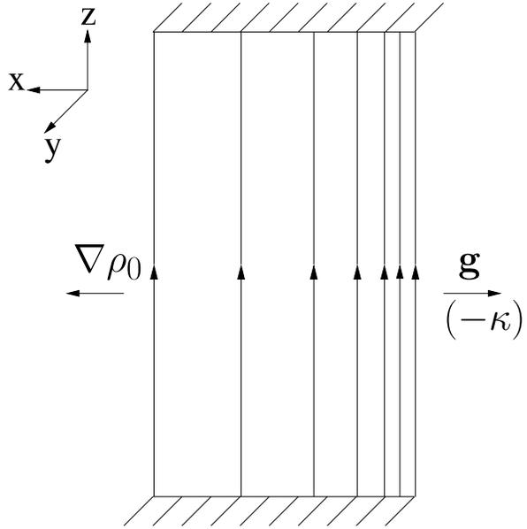
FIG. 1: A shearless slab configuration of line-tied flux tubes. The gravity  $\mathbf{g}$  here is equivalent to the magnetic curvature  $-\kappa$  in a curved magnetic configuration.
