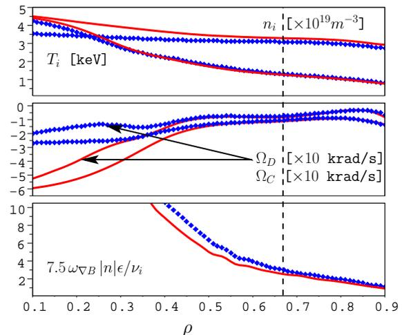
FIG. 1: (top, center) NCLASS plasma profiles for shot 138574 at  $t = 1900$  ms (solid line) and  $t = 2400$  ms (marker). Vertical dashed line shows surface where CER feedback was performed. (lower) Plot indicating  $\nu_i/(|n|\epsilon) < 7.5|\omega_{\nabla B}|$  over most of the plasma profile and thus the peak NTV torque is governed by the sbp regime [17] until  $\rho \geq 0.8$  where the sbp and  $1/\nu$  [15] regimes become comparable in this model.
