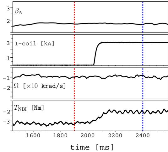
FIG. 2: Experimental time trace for shot 138574, showing  $\beta_N$ , I-coil current, rotation rate at  $\rho = 0.67$ , and the total injected neutral beam torque. Positive rotation and NBI torque are both in the co- $I_p$  direction. Vertical dashed lines refer to the profiles plotted in Fig. 1 before ( $t = 1900$  ms) and after ( $t = 2400$  ms) I-coil switch-on.
