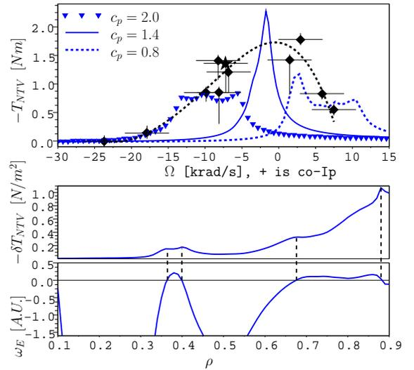
FIG. 4: (top) Total cylindrical ( $m, n = 2, 3$ ) NTV torque integrated over the plasma profile as a function of  $\Omega$  at  $\rho = 0.67$ ; symbols are as in Fig. 3. Varying only the poloidal rotation value,  $c_p$ , the best fit is  $c_p = 1.4$  (solid line) bracketed by two other curves with  $c_p = 1.4 \pm 0.6$  respectively. Representative torque density (center) for  $c_p = 1.4$ , which has local maxima where  $\omega_E \approx 0$  (lower plot) and indicated with vertical dashed lines.
