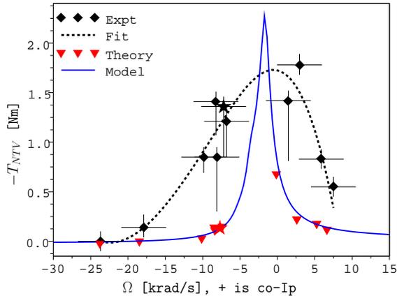
FIG. 3: Comparison of measured NTV (diamonds), and cylindrical torque model (line) versus deuterium toroidal rotation rate (obtained from NCLASS) at  $\rho = 0.67$ . A least-squares spline fit (dashed) is shown for the data. Individual NTV torque points (triangles) are shown for each shot by taking the average of (7) computed slightly before and after I-coil switch-on. The starred points indicate shot 138574.
