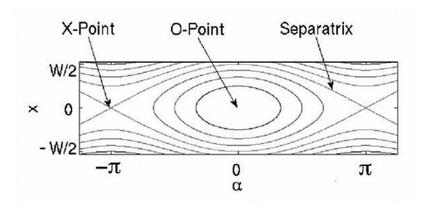
FIG. 1. Contours of  $\Psi^*$ , plotted in  $(x, \alpha)$ .
